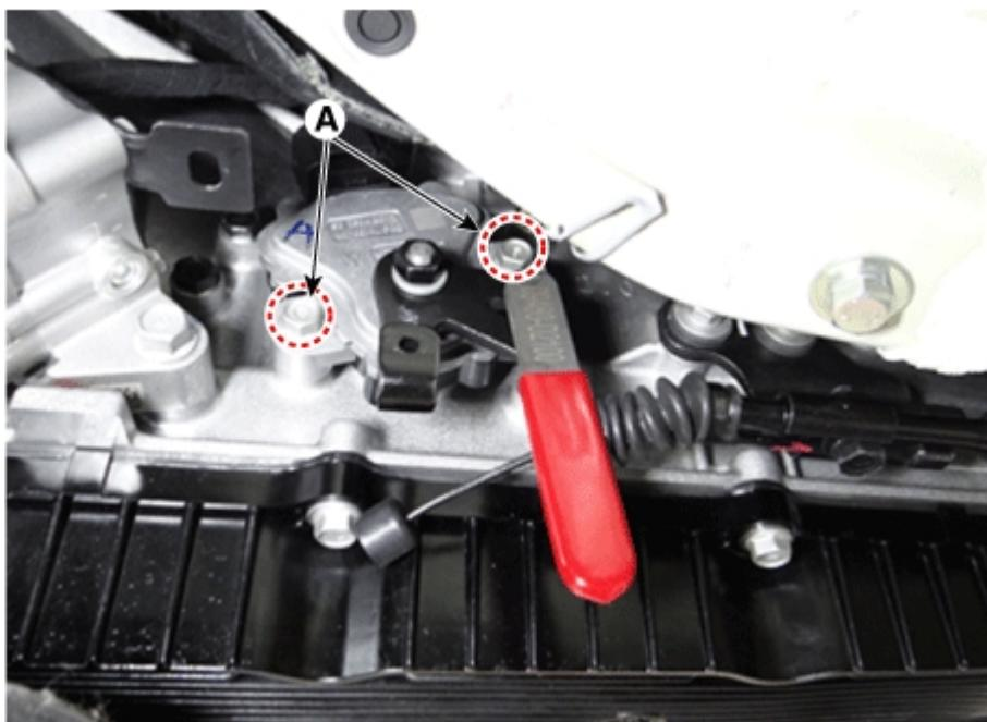
5. Tighten the parking release lever mounting nut (A).
