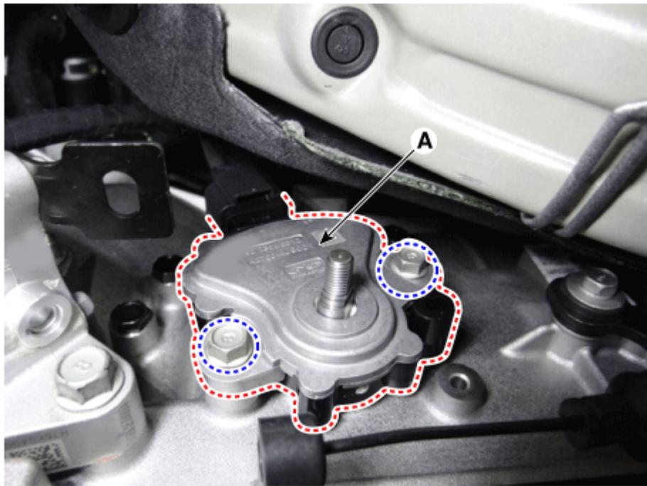
4. Disconnect the parking switch connector (A).
