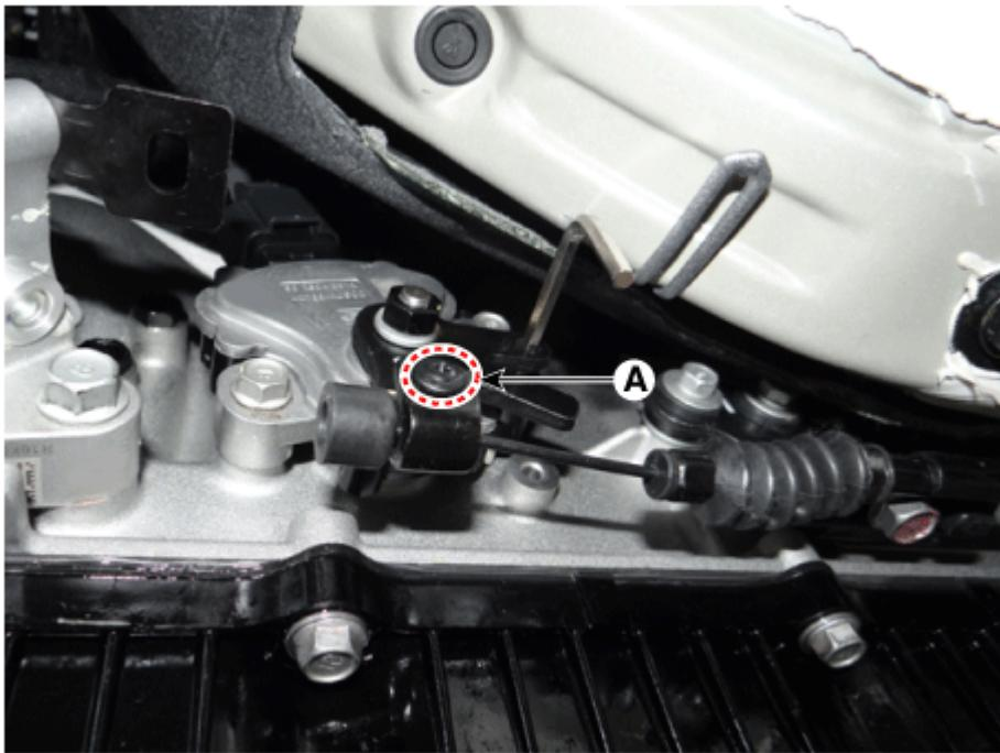
2. Remove the parking release lever (A) after loosening the nut.
